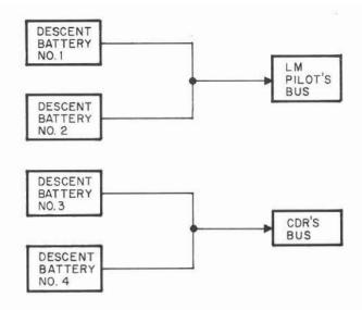
Later in the mission, the LM will be staged, separating the descent and ascent stages. To maintain power on the two DC busses, two batteries located in the ascent stage are connected to the busses. In normal operation, each bus is connected to one battery, but in the event of abnormal operation, the battery may also be connected to the other bus.
