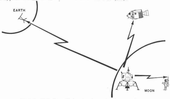
To accomplish these links, two Communications sections are utilized; S-Band for long range link, and VHF for the short range link.
