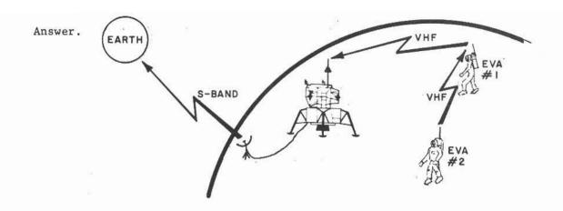
Up to this point, the majority of the signals discussed have been voice and ranging. The MSFN can also receive LM telemetry signals. The S-Band section transmits high-bit-rate (HBR) or low-bit-rate (LBR) telemetry. The telemetry information tells the Flight Controller the status of the LM.
